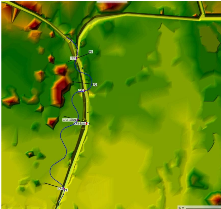
Figure 4.3. Existing digital terrain model with the location of control points CP's and cross sections "P".
